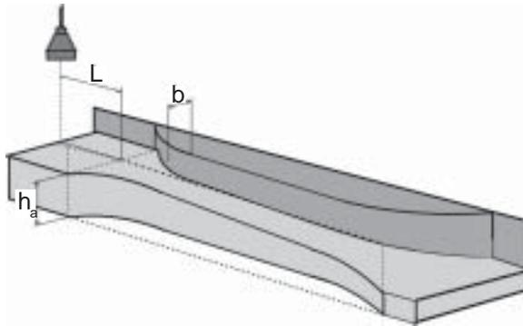
713 follows the calculation method for long throated Venturi flumes described in ISO 1438. The connection between level and flow is complex and can not be described in a simple formula. When dimensioning the following simplified formula can be applied.
