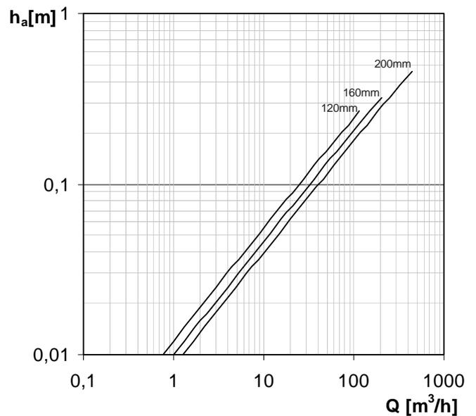
Q/h diagram for the Khafagi Venturi flumes, the height h<sub>a</sub> is shown as a function of the flow Q.
