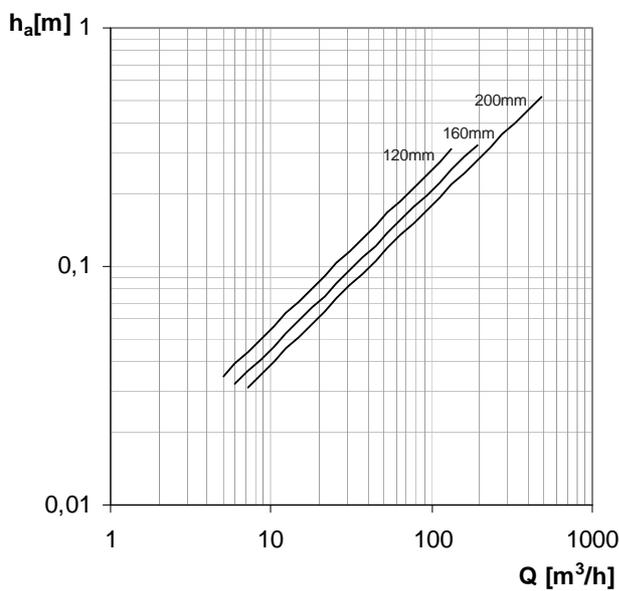
Q/h diagram for the long throated Venturi flumes, the height h<sub>a</sub> is shown as a function of the flow Q.
