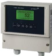
The 7200 Monitor combines with the Partech range of Suspended Solids and Turbidity Sensors to give a cost-effective solution to measurement of Suspended Solids, Turbidity and Sludge Density. The Monitor provides a large character display of the measured value combined with a scrolling information bar showing measurement status.
