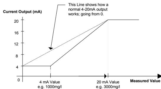
Figure 19 Example output configuration (4-20mA)
