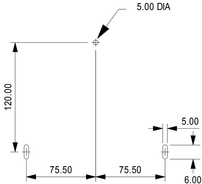
Figure 2 7200 Field Mount mounting hole positions
