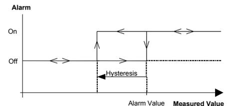
Figure 18 High Alarm with hysteresis
