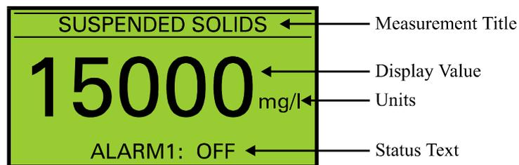
*Figure 5 Measure Mode Display*
